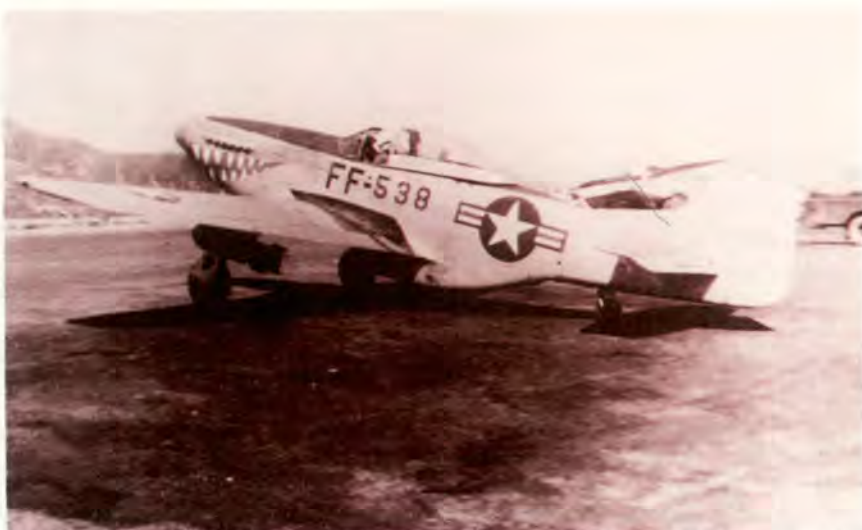
The P-51 Mustang was a formidable fighter in WW II, but it was rapidly being outmoded in the new jet age of 1950. However, with a combat range of up to 1,000 miles, six .50 caliber machine guns, and other ordnance, the Mustang was still effective.
